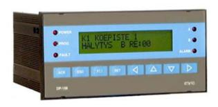
The DP-158 is a programmable 8, 16 or 32 channel measurement and alarm centre. In addition to measurement inputs the centre has inputs for 8 relay contact circuits. In addition to, the actual measurement and alarm operation, the centre is equipped with memory storage, inhibit, control, and report functions.
