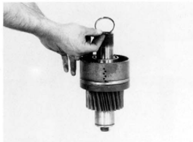
Figure 91 Remove inner and outer bearing spacer.
