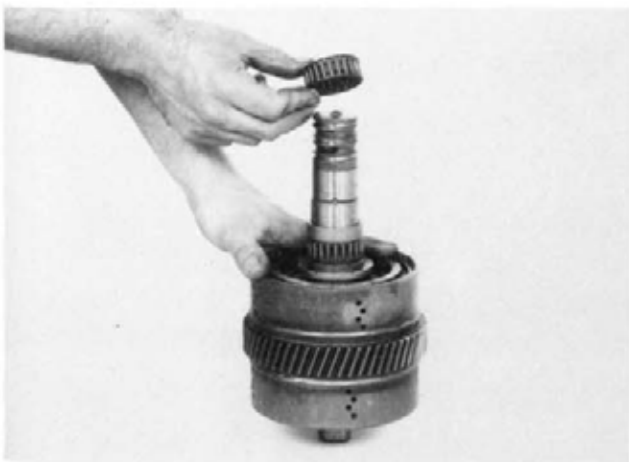
Figure 165 Remove clutch gear outer bearing.
