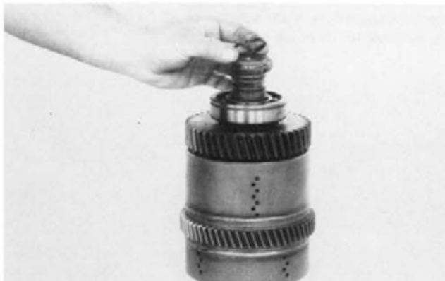
Figure 158 Install clutch shaft oil sealing rings. Grease rings to facilitate reassembly into front housing.
