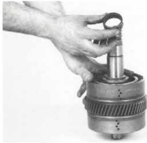
Figure 202 Install clutch gear inner bearing.
