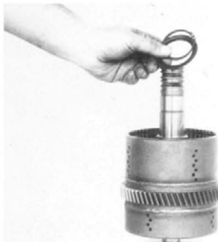
Figure 126 Compress piston return springs (Belleville washers). Remove return spring retainer ring and ring retainer.
