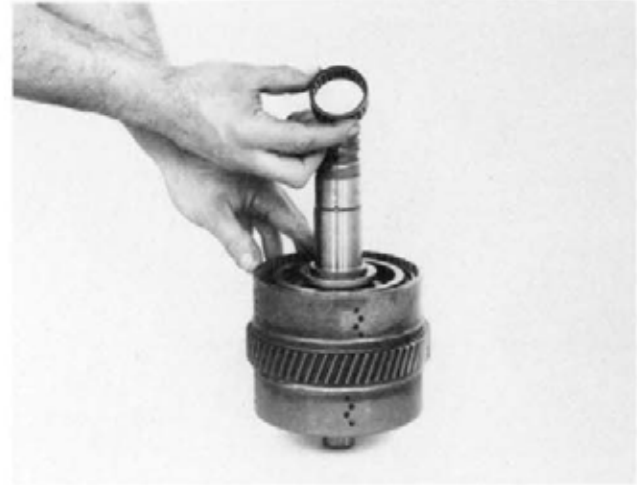
Figure 167 Remove inner bearing.
