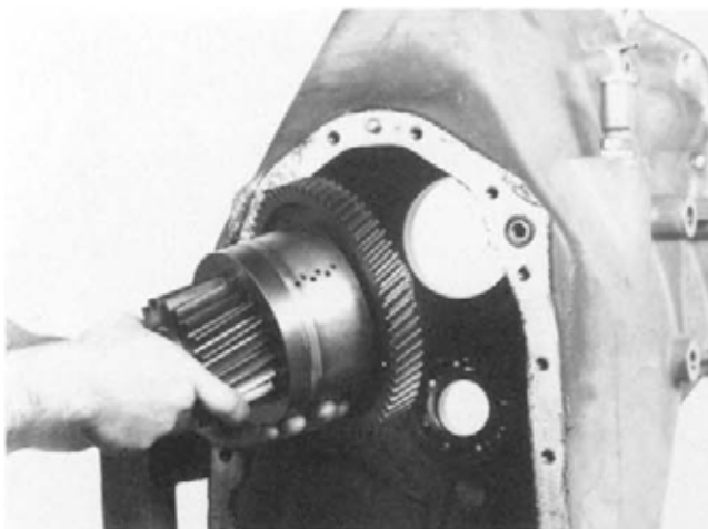
Figure 54 Remove 1st speed clutch assembly.
