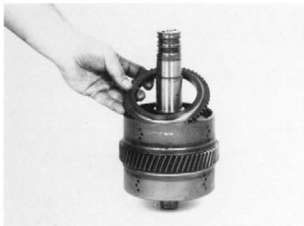
Figure 172 Remove end plate.
