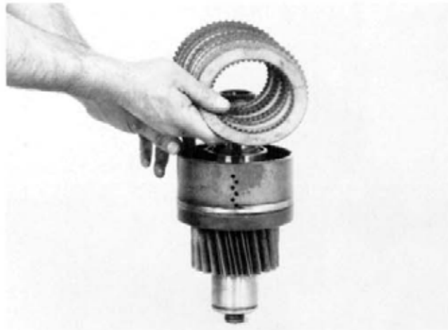
Figure 90 Remove inner and outer clutch discs.
