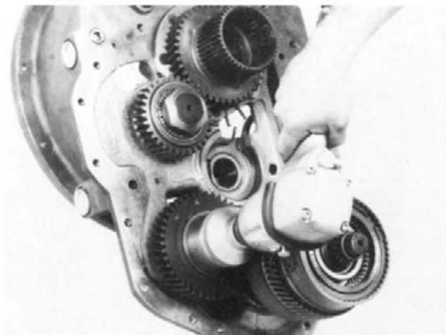
Figure 66 Unclinch lock nut by straightening upset metal in notch in idler shaft. Remove shaft nut.
