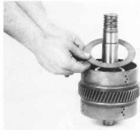
Figure 196 Install one friction disc. Alternate steel and friction discs until the proper amount of discs are installed. First disc next to the piston is steel, last disc installed is friction.
