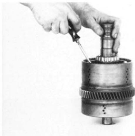
Figure 122 Remove clutch end plate retainer ring.
