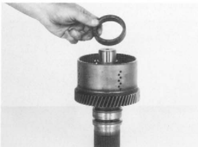
Figure 216 Remove piston spacer.
