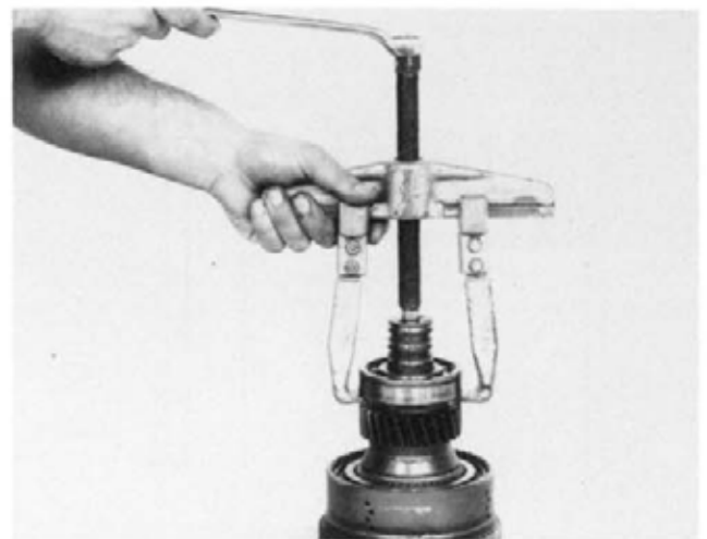
Figure 161 Remove front bearing.
