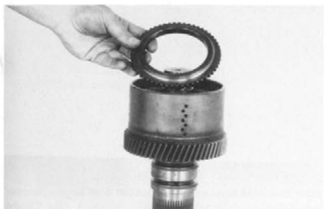
Figure 212 Remove end plate.
