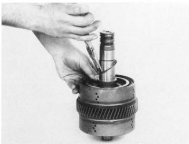
Figure 170 Remove thrust washer locating ring.
