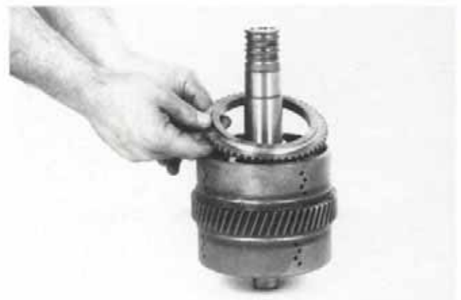
Figure 197 Install end plate.
