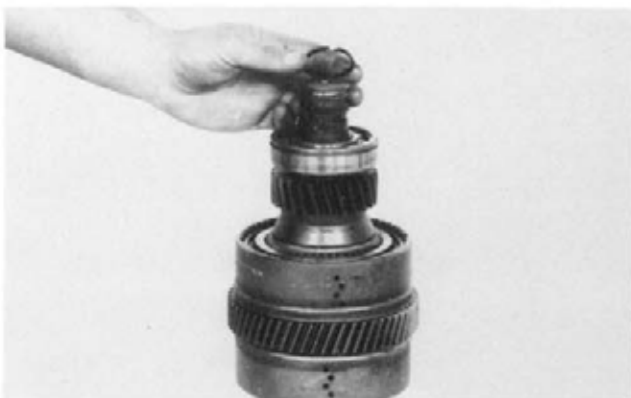
Figure 159 Remove clutch shaft oil sealing rings.
