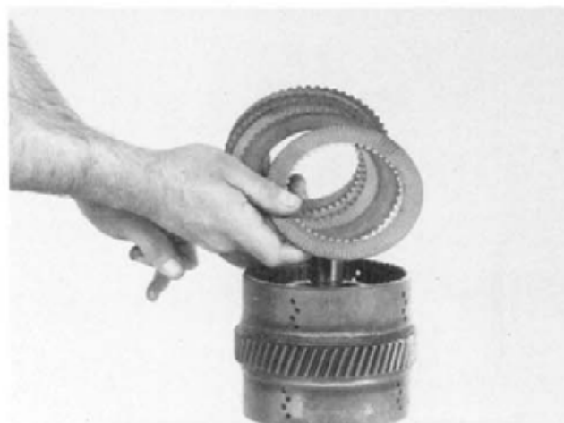
Figure 179 Remove inner and outer clutch discs.
