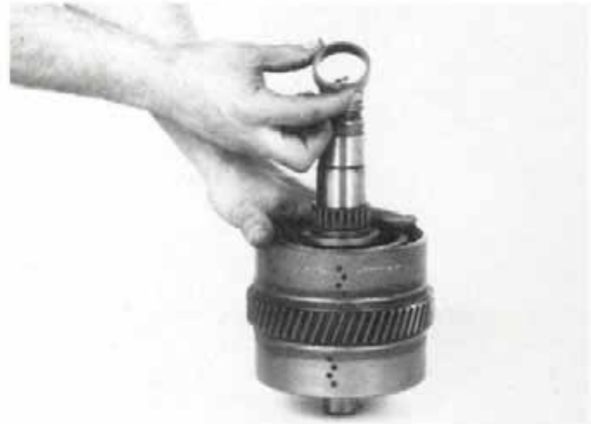
Figure 203 Install bearing spacer.
