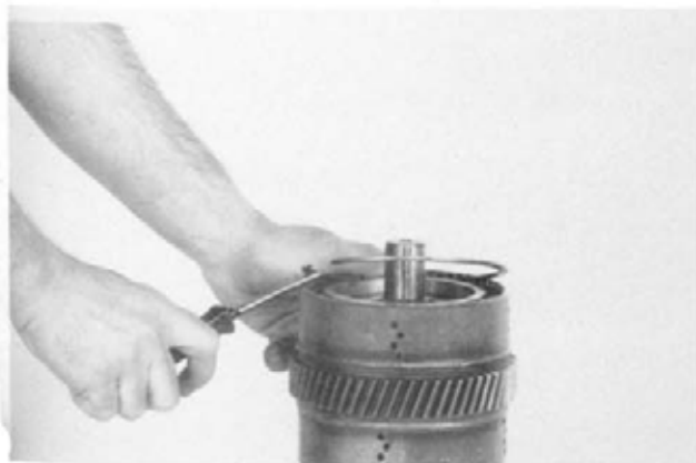
Figure 177 Remove end plate retainer ring.
