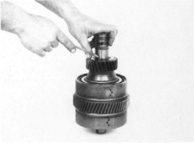
Figure 163 Remove thrust washer lock ball.
