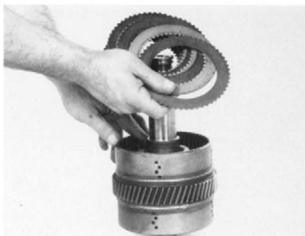
Figure 173 Remove inner and outer clutch discs.
