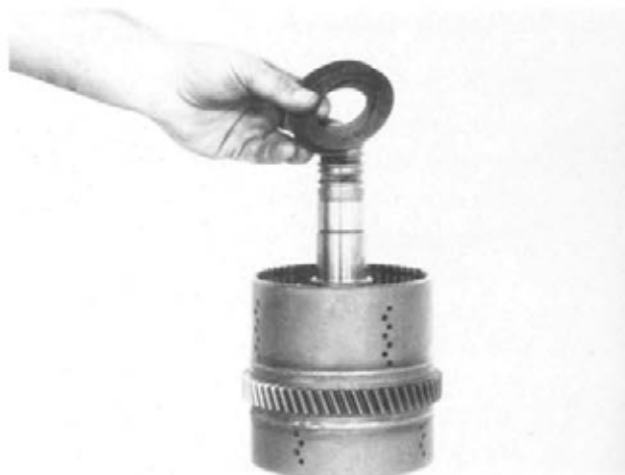
Figure 127 Remove piston return springs. (Belleville washers.)
