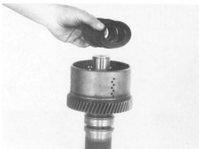
Figure 215 Remove piston return springs. (Belleve washers).
