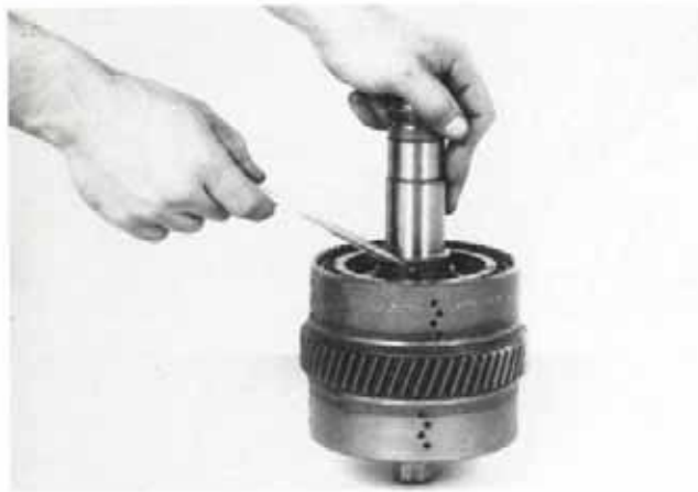
Figure 200 Position lock ball in hole in shaft. A small amount of grease will hold ball in place.
