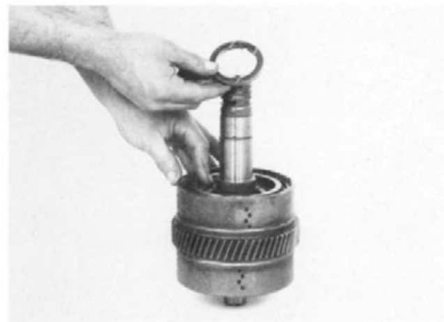
Figure 168 Remove gear rear thrust washer.
