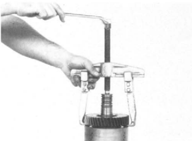
Figure 121 Remove reverse gear and bearing spacer.
