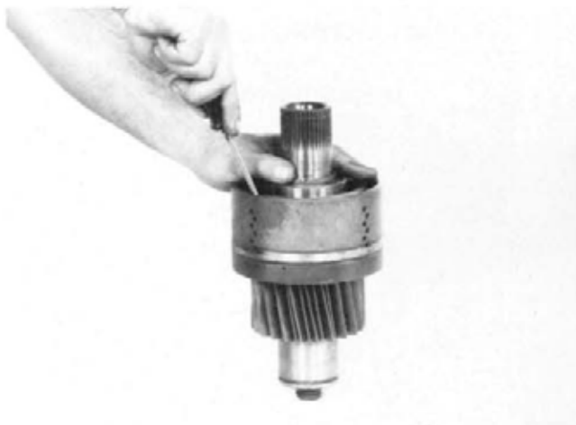
Figure 88 Remove clutch disc end plate retainer ring.
