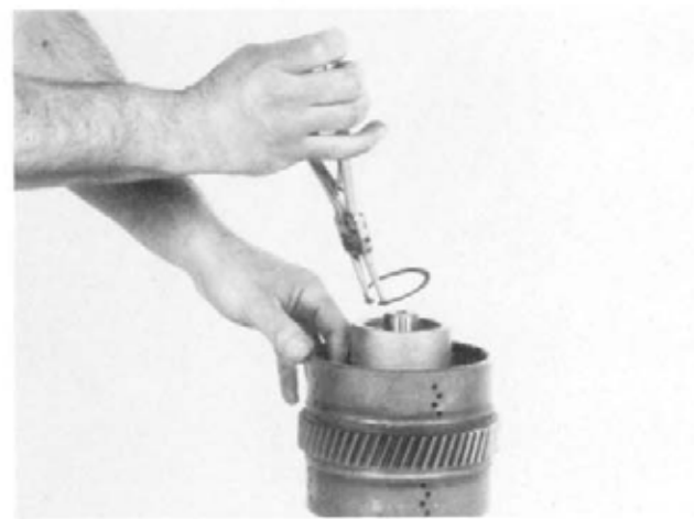
Figure 180 Remove return spring retainer ring.
