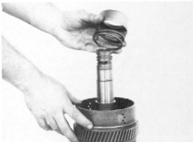
Figure 175 Remove spring retainer and spring.
