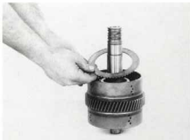
Figure 195 Install one steel disc.
