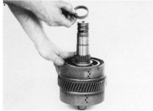
Figure 166 Remove bearing spacer.
