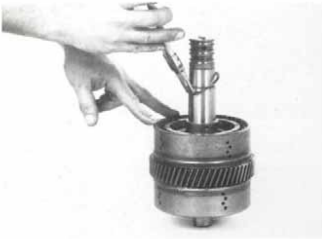
Figure 199 Install inner thrust washer locating ring.
