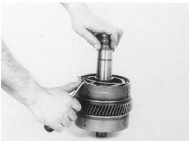
Figure 171 Remove clutch disc end plate retainer ring.
