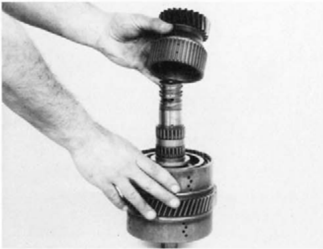
Figure 164 Remove clutch gear and disc hub.
