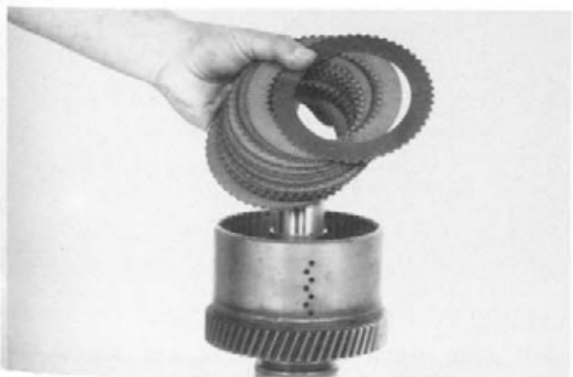
Figure 213 Remove inner and outer clutch discs.
