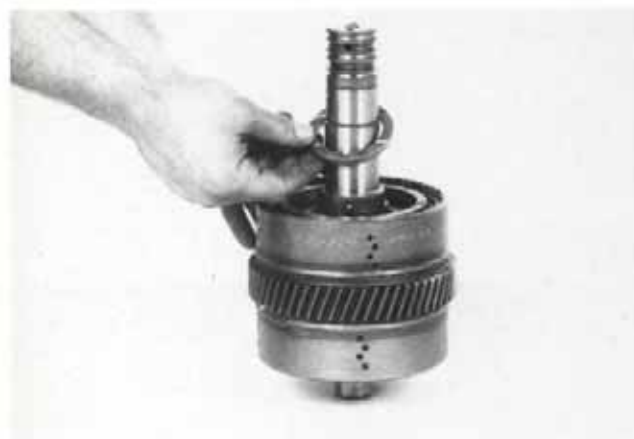
Figure 201 Position inner thrust washer on shaft aligning notch in washer with lock ball.
