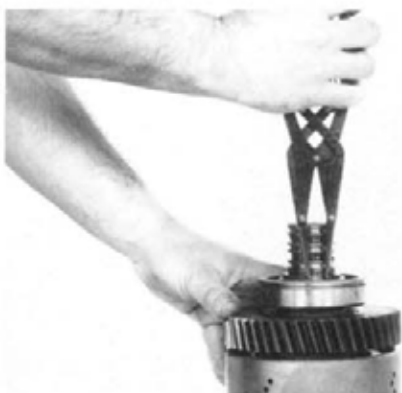
Figure 117 Remove front bearing retainer ring.
