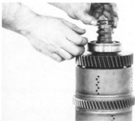
Figure 116 Remove clutch shaft oil sealing rings.
