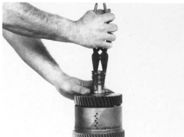
Figure 119 Remove clutch gear bearing retainer ring.
