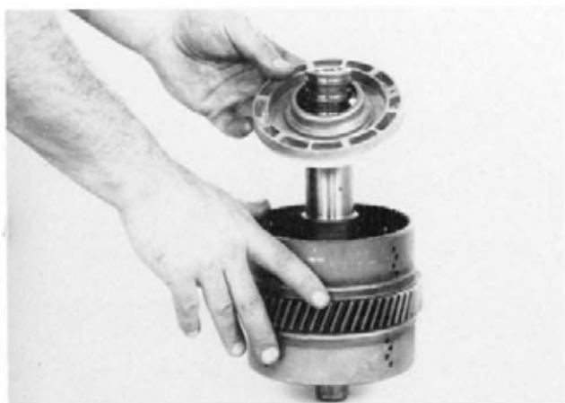
Figure 176 Remove clutch piston.
