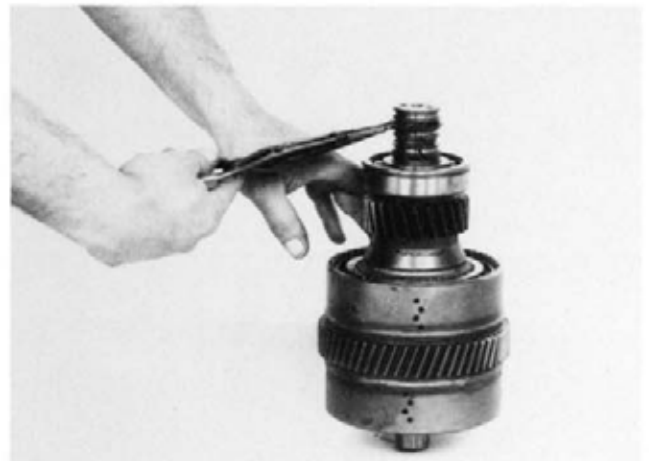
Figure 160 Remove front bearing retainer ring.
