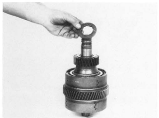
Figure 162 Remove gear front thrust washer.
