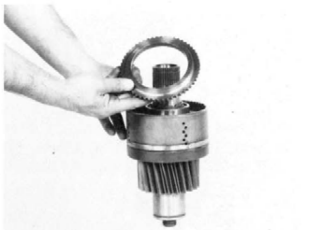
Figure 89 Remove end plate.
