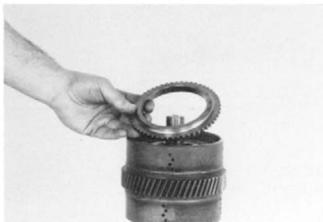
Figure 178 Remove end plate.
