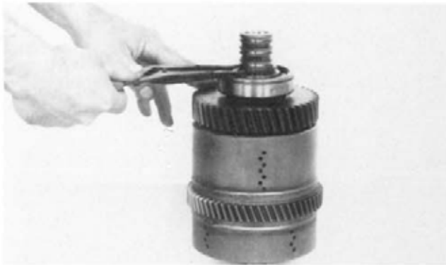
Figure 157 Install front bearing retainer ring.
