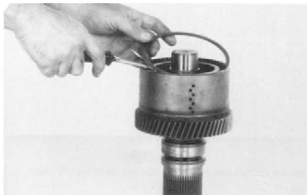
Figure 211 Remove clutch disc end plate retainer ring.
