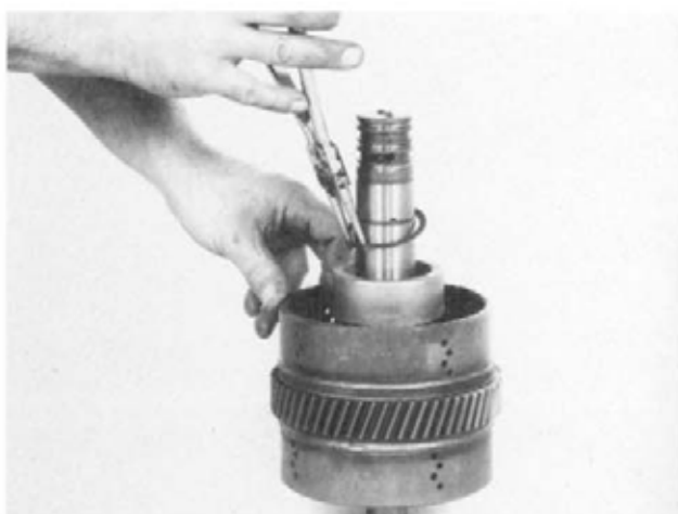
Figure 174 Remove clutch disc return spring retainer ring.
