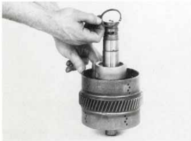
Figure 194 Compress return spring and install spring retainer ring.
