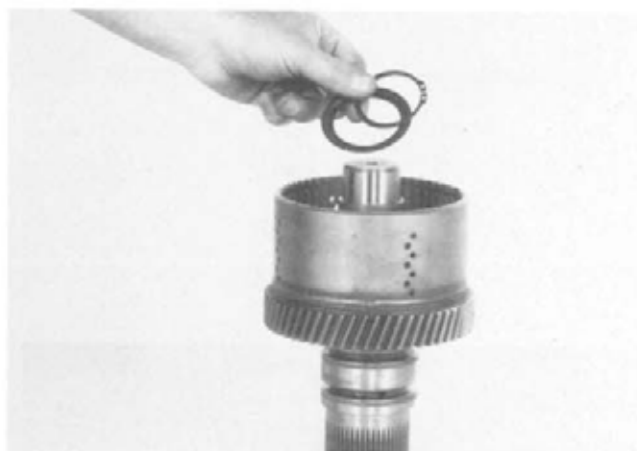
Figure 214 Compress piston return springs (Belleve washers). Remove return spring retainer ring and ring retainer.
