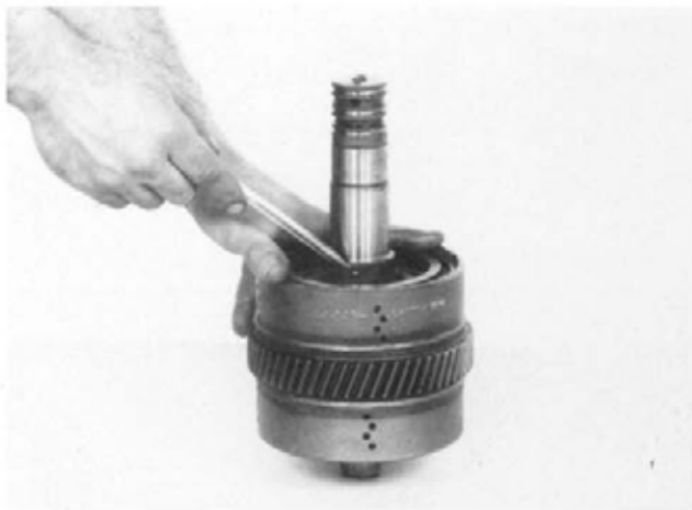
Figure 169 Remove thrust washer lock ball.
