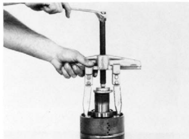
Figure 92 Remove low gear inner bearing.
