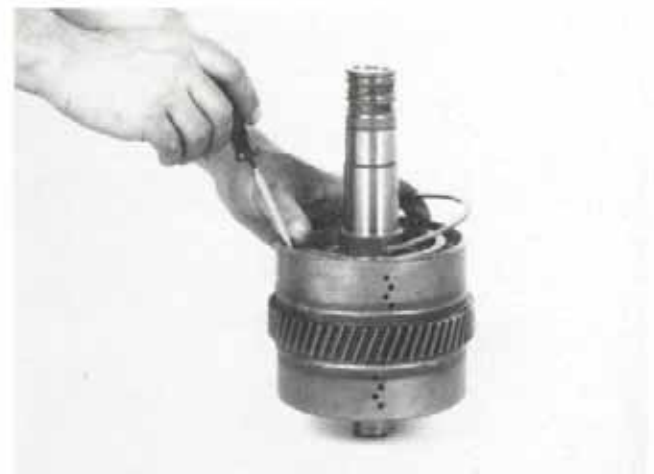
Figure 198 Install end plate retainer ring.
