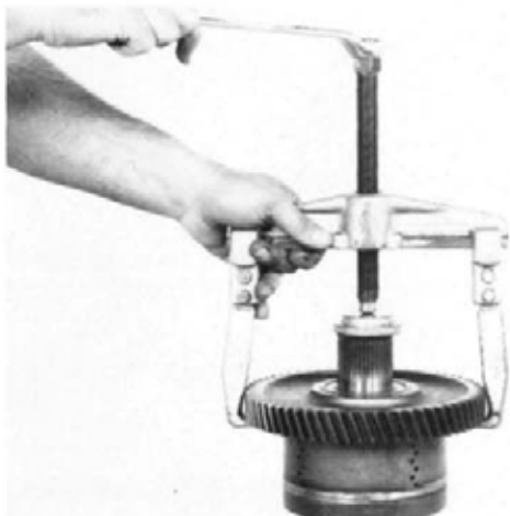
Figure 87 Remove low gear and outer bearing.
