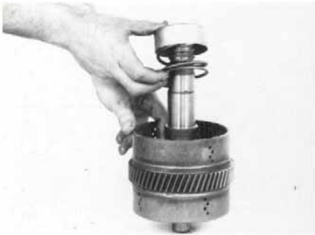
Figure 193 Position return spring and spring retainer on clutch shaft.
