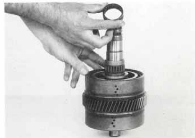
Figure 204 Install outer bearing.
