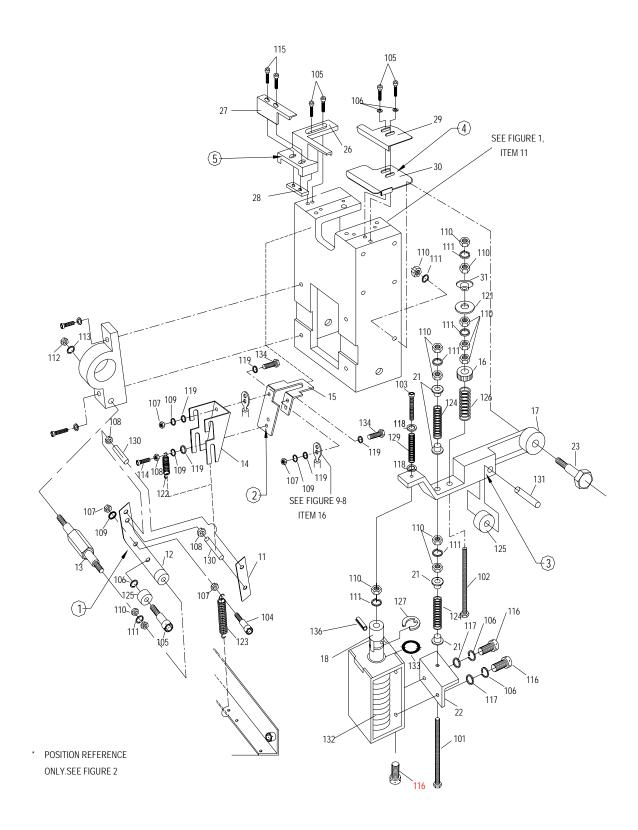
FIGURE 5.HOT-KNIFE AND TENSION LEVER ASSEMBLIES
