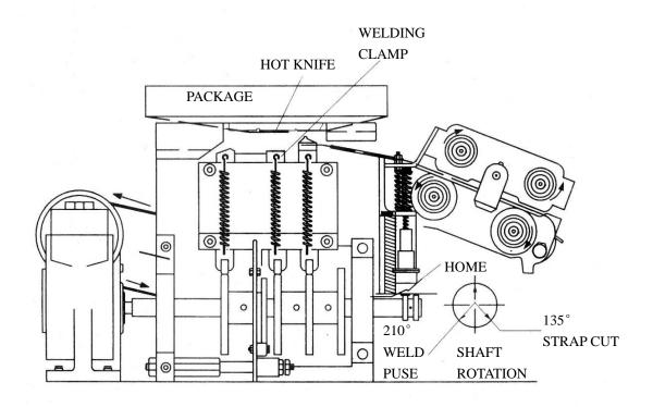
FIGURE 17. STRAP IS CUT & WELD IS MADE
