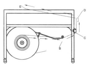
FIGURE 9. STRAP THREADING DIAGRAM
