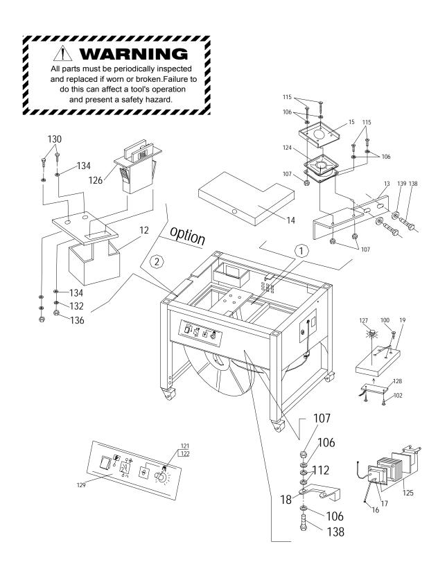
FIGURE 9-5.ELECTRICAL COMPONENTS
