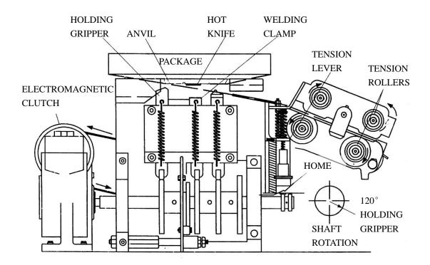
FIGURE 16. HOLDING GRIPPER AND HOT-KNIFE
