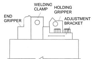
PAETS SEEN FROM REAR SIDE HEAD FIGURE 22. WELDING CLAMP AND GRIPPER CLEARANCE
