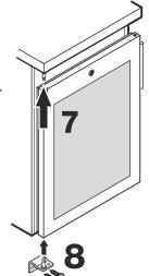
**8.** Insert hinge bracket in lower door mounting and screw into place.
